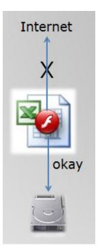
We embed a Flash object in an Office document. This flash object is allowed to access local files, and not allowed to access internet. However there is a problem when handling the 'mms' protocol. When the flash object opens an mms link, IE will be launched, and then media player will also be launched (by IE) as well. The media player will connect to the link.
