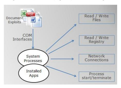
Not only defeating HIPS, the approach could also defeat automation analyzing sandbox system. The malware 'process' actually does nothing directly. The sandbox could record nothing if the sandbox only tracks malware process.
