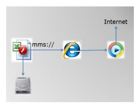
Using this flaw, we could retrieve user information, and use mms protocol to send information to internet. For example, we might steal user's cookie, user's saved password, etc. And we could use this technique to probe user environment.
