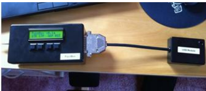
Figure 7 – Fuzzbox -the Arduino-based USB fuzzer
