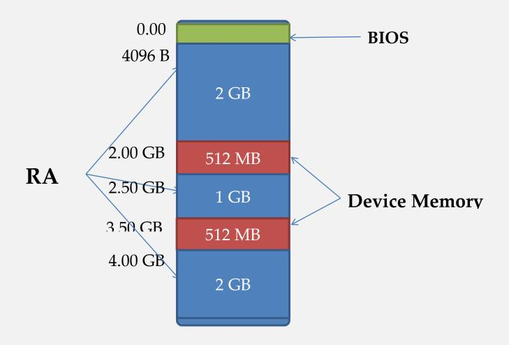
The figure above is a representation of the physical memory as seen by the processor. Blue blocks are the RAM.
