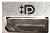
Figure 5: DisplayPort socket (The DP++ logo indicates dual mode i.e. compatible with DVI/HDMI displays)
