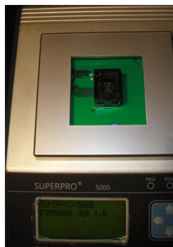
Figure 2 Extracting NAND Flash Data using a XELTEK SuperPro 5000
