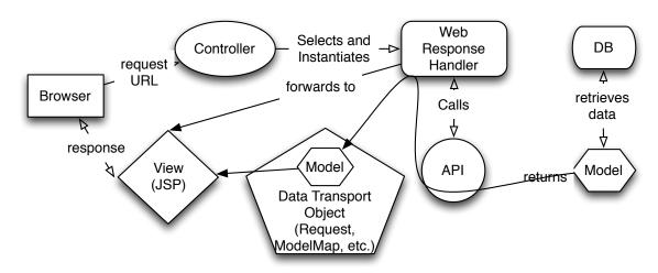
The controller (represented by the controller oval and web response handler) receives input from the user, retrieves or sends data from or to the model and invokes the view. The model is responsible for holding the state of objects that are presented by the view. The View is responsible for rendering the model in a specified presentation format.
